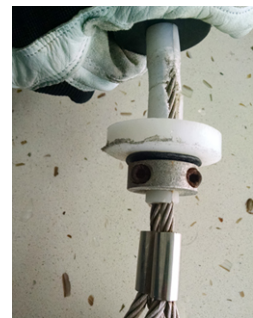
Broken Cable Sleeve
