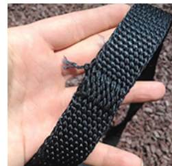
Broken Strand in Slotted Webbing
